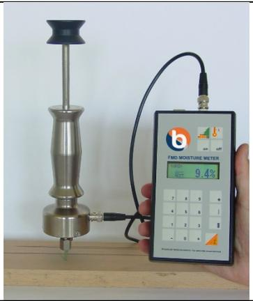
A hand holds the FMD6 moisture meter, which is connected to a probe inserted into a piece of wood. The device's screen displays a moisture reading of 9.4%. |
